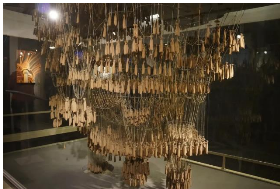
Figura 1 – Modelo de cordas e pesos – fonte: https://parametric-architecture.com/la-sagrada-familia-gaudis-chain-model/?srsltid=AfmBOoqtBhbknZgDG_QXaqXse9yPDZ18fpj3wZVUT-eSdsF0I989r0Lj
