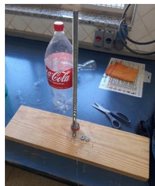
Figure 1: Apparatus used to cut the plastic strips (Source: Self)
