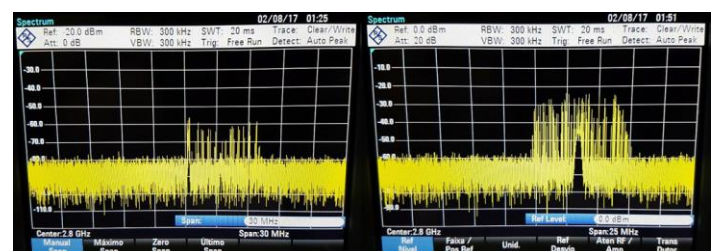
Image 5. Measured PSD (a) with antenna (b) with cable.
