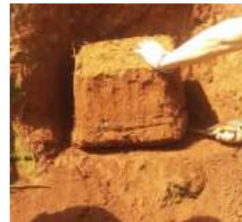
Image 1. Withdrawal of undisturbed soil sample
