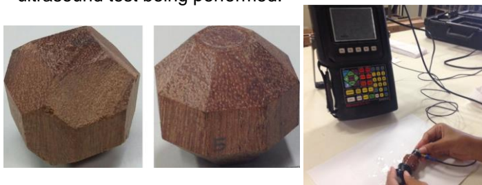
Image 1. Polyhedron of 18 and 26 faces (a) and ultrasound test (b).
