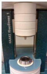
Figure 1. Rheometer used in the experiment
