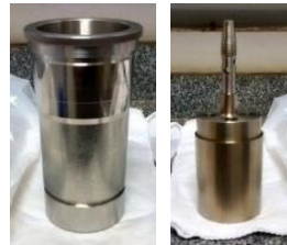
Figure 2. Cylindrical parts used to simulate the shaft and the bearing
