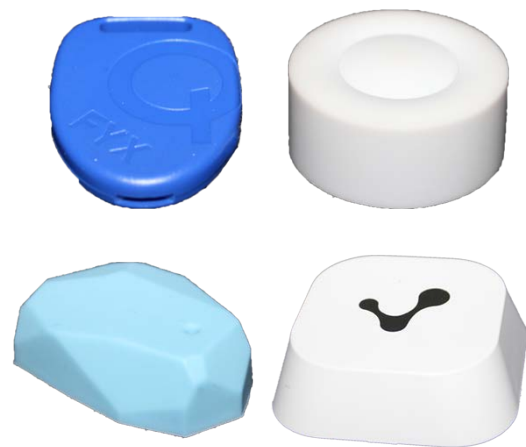
Figure 1. Beacons tested during the development. Models: Gimbal Series 10, Minew MS54V3, Estimote and Kontakt.io, respectively, from left to right and from top to bottom.
