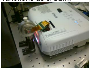
Image 2. Detail of the experimental setup: the LCD screen connected to the Datashow.
