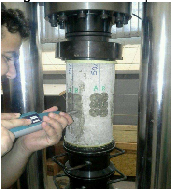
Image 1. Sclerometric impact test.
