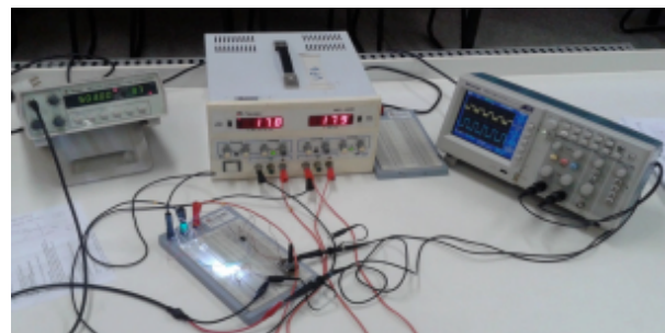
Figure 1. Protoboard-mounted circuit, power supply, function generator and oscilloscope.
