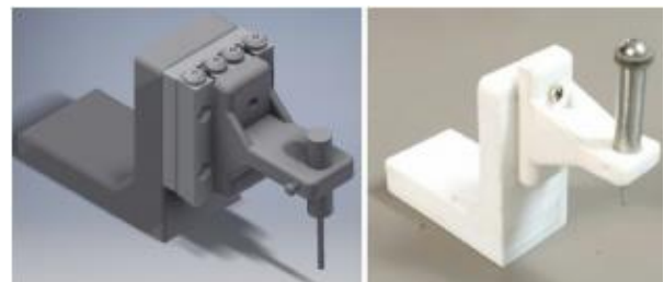
Figure 1: System prototype for measure automation in the Z direction. On the left, the pre-production, a CAD drawing of the prototype. And on the right, the 3D printed prototype without the piezo positioner.
